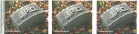
Figure 1.4 JPEG compression is a lossy format. Nearly every digital camera can save images in the JPEG format. JPEG files degrade when repeatedly added and saved. The JPEG format is also used by the image compression algorithm in Adobe PDF documents.
